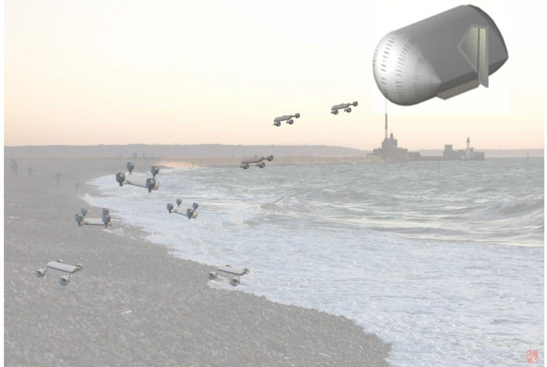
the Hybrid Advanced Mobility Propulsion System (HyAMPS™) (US Patent 10,180,083, additional patents pending). Using a set of actuators, the HyAMPS™ can act as a ducted fan propeller in air or water or engage the ducted shroud to serve as a wheel on any surface. Actuation of the motion arms and steering system allows forward (or backward) thrust, vertical thrust and steering in any medium.
